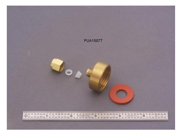
The **Twist Bottle Adapter** provides the means to install a **Sentry** temperature probe into a bottle with a twist-off closure for a test.
